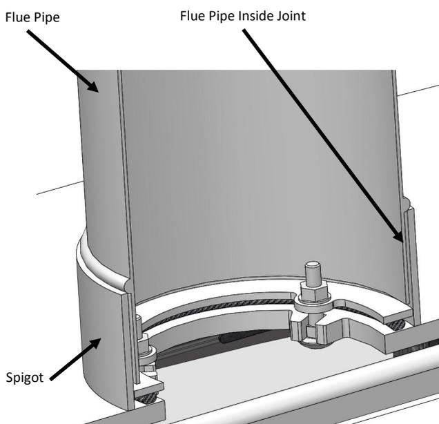
Figure 2: Fitting the flue pipe inside the spigot collar.
