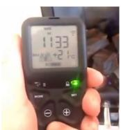
To adjust high and low whilst holding the handset and green light on press + & - to adjust for the preferred heat setting.
