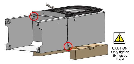
STEP 5: Taking care, return the appliance and accessory to the upright position. Extra caution will be needed as the centre of gravity will have moved by fitting this new accessory.
