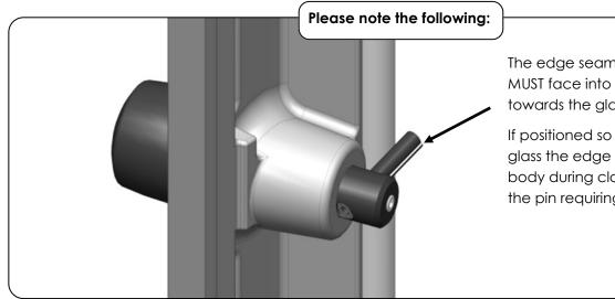
The edge seam of the scroll pin MUST face into the fire box NOT towards the glass.
