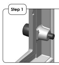
Insert the door shaft through the hole in the door.
