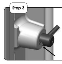
Do not drive the pin further than the back face as it will impede the free rotation of the handle assembly.
