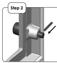
Ensuring the seam of the pin is facing away from the glass. Tap the scroll pin into the pin hole on the shaft until flush with the back face of the pin hole drilling.
