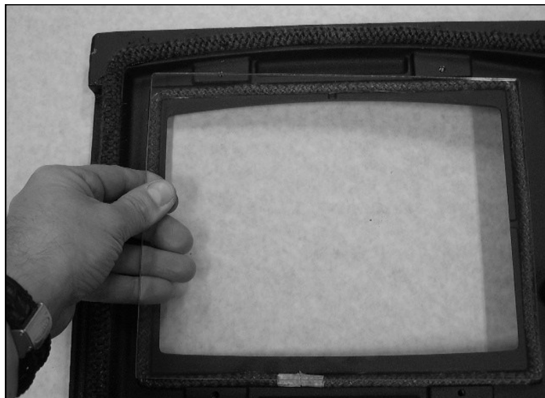
Fig. 10. Positioning The Glass
